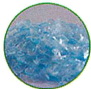
PET Bottle Flakes Used as Raw Material
